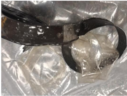
Microfilm damaged by vinegar syndrome
