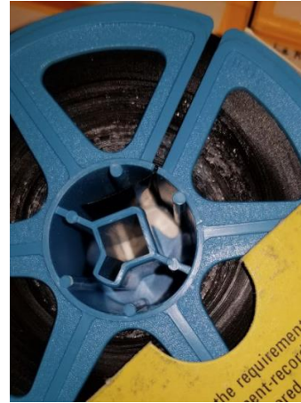
Microfilm damaged by vinegar syndrome
